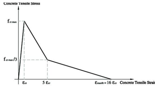
Fig. 10: Tension-softening curve proposed by Massicotte et al. [48].
