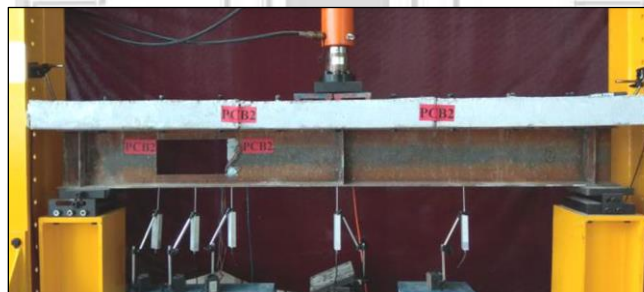
Fig. 3: The 50-ton hydraulic testing machine [40].
