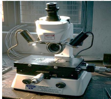
Fig.1 Toolmaker microscope (30× magnification) quantifying HSS flank wear V_b after standardized 150 mm axial cut length. Scale: 0-0.5 mm.
