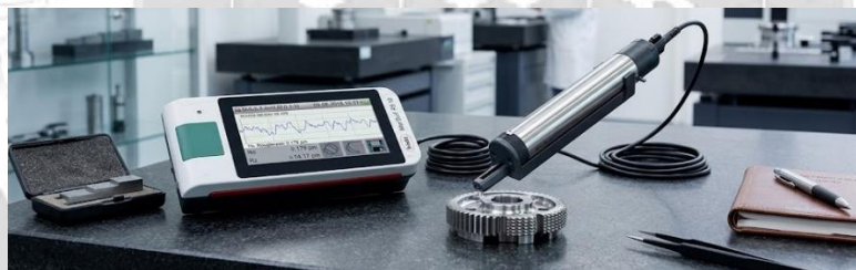
Fig.2 Mitutoyo SJ-210 portable surface roughness tester measuring arithmetic average R_a . Three-line protocol (machine-left, center, machine-right) averaged per ISO 4287. Range: 0-3 \mu\text{m} ( \pm 0.5 \mu\text{m} )
