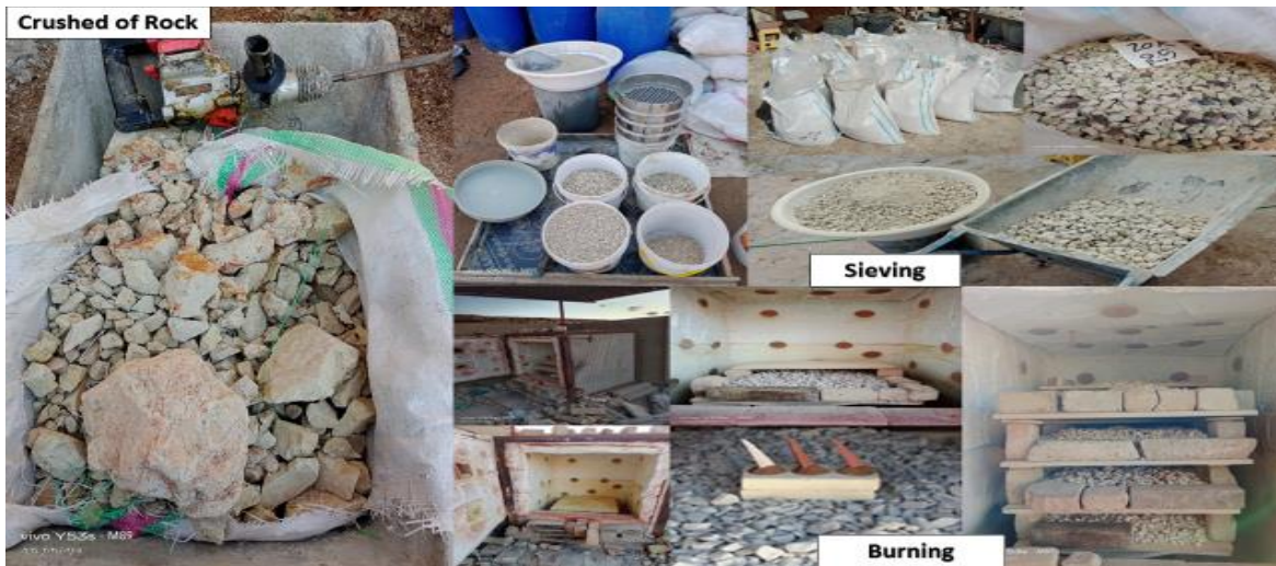
Fig. 1: Production Step of Attapulgite Lightweight Aggregates
