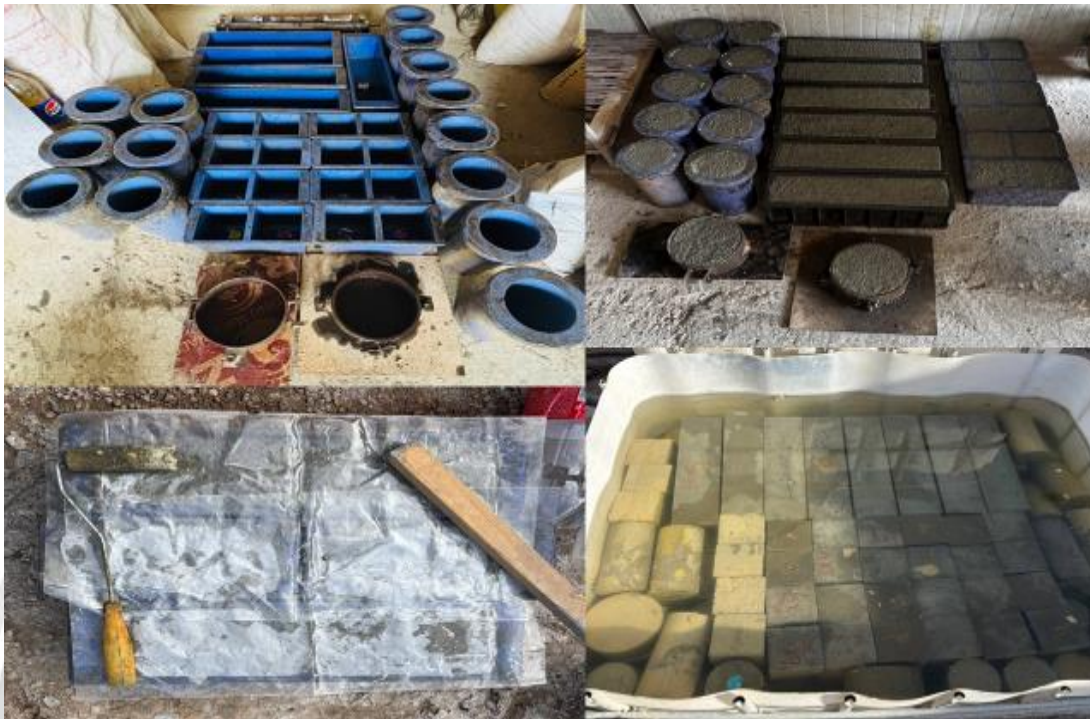
Fig. 4: Casting and Curing of LWSCC mixture
