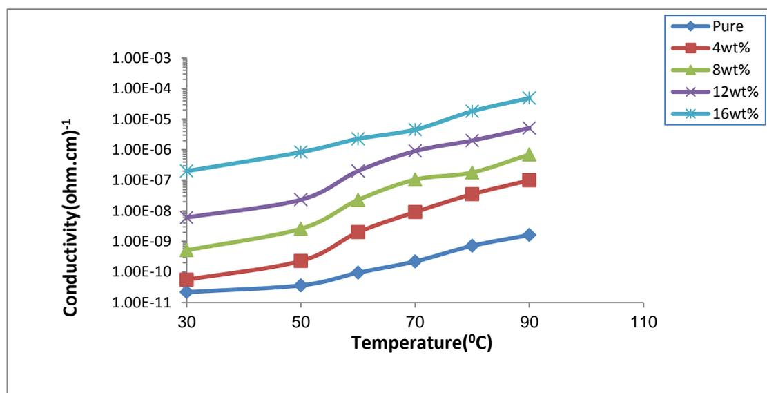
Figure 3: Variation of D.C. electrical conductivity with temperature for (PVA-Al<sub>2</sub>O<sub>3</sub>)nanocomposites
