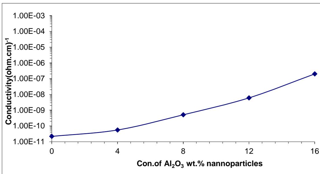
**Figure1:Variation of D.C electrical conductivity with Al<sub>2</sub>O<sub>3</sub> concentration wt.% for(PVA-Al<sub>2</sub>O<sub>3</sub>) nanocomposites at room temperature."**
