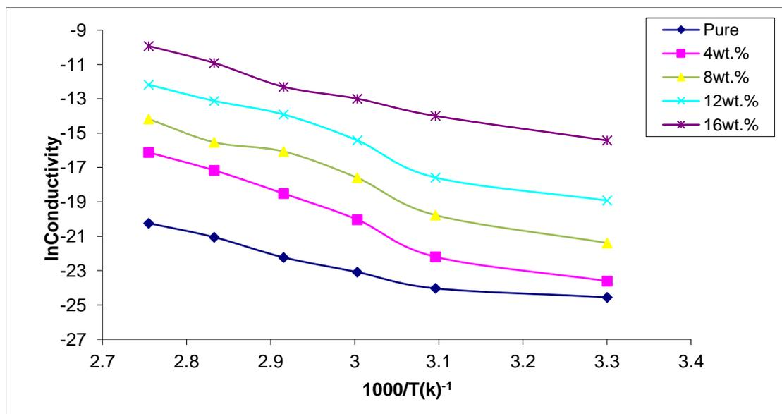
**Figure 4: Variation of D.C. electrical conductivity with reciprocal absolute temperature for (PVA-Al<sub>2</sub>O<sub>3</sub>) nanocomposites.**
