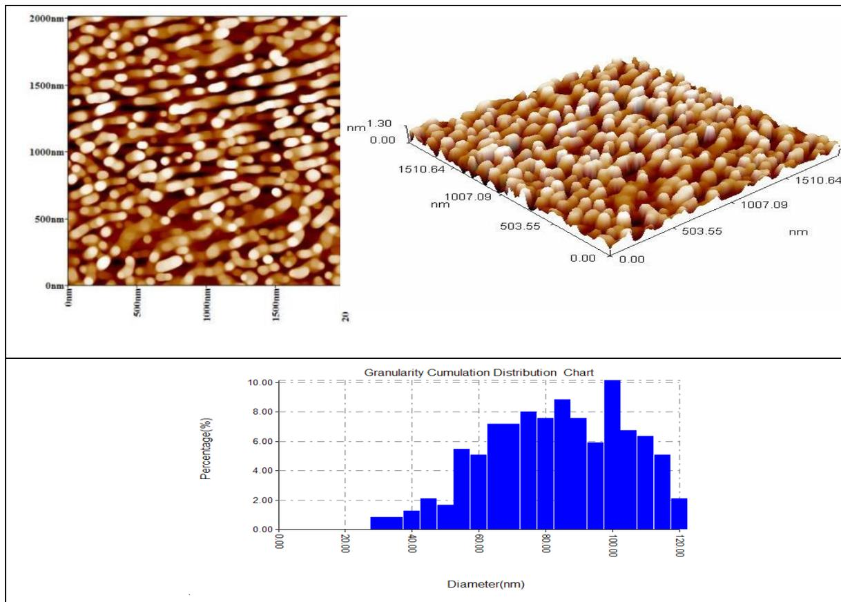
**Figure (3). 2-D, 3-D dimensional AFM image and the granularity accumulation distribution chart of TiO<sub>2</sub> powders with annealing temperature at 400°C for 120 min.**
