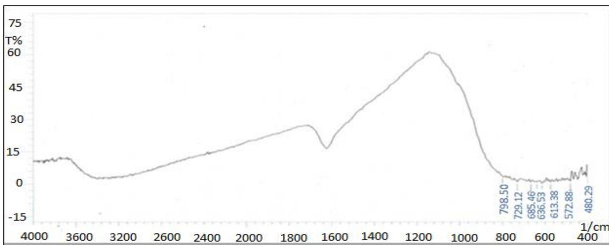
**Figure (2). FTIR transmittance spectrum of  $\text{TiO}_2$  annealing at  $400^\circ\text{C}$  for 120 min.**
