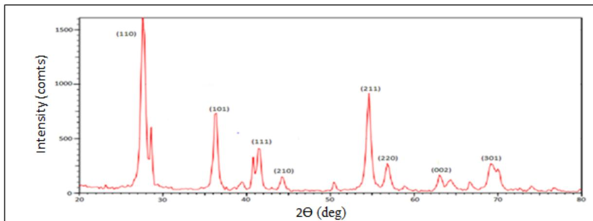
Figure (1). XRD patterns of TiO<sub>2</sub> annealing temperature at 400°C for 120 min.
