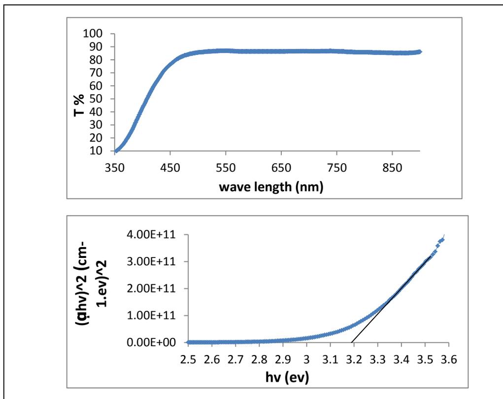
**Figure (5). Optical Transmission as a function of wavelength for r-TiO<sub>2</sub> annealing at 400 °C for 120 min.**
