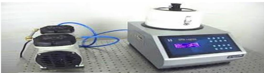
**Figure. (1): Spin coating system with its control.**
