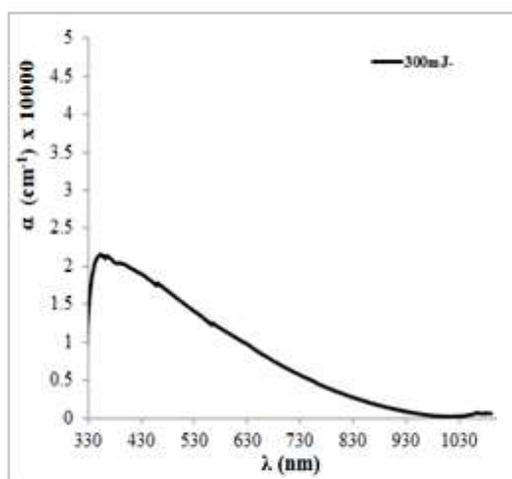
Fig. 6 The absorbance spectra for DLC film at 300mj
