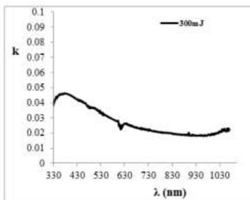
Fig. 8 Extinction Coefficient for DLC thin film at 300 mj.
