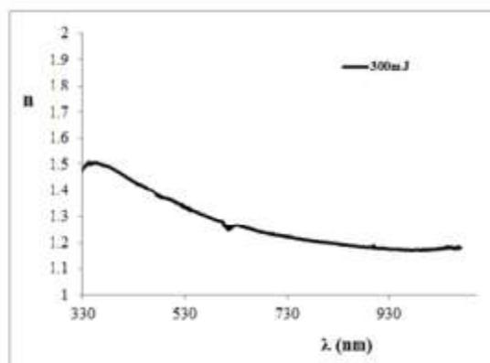
Fig. 9 Refractive index for DLC thin film at 300 mj
