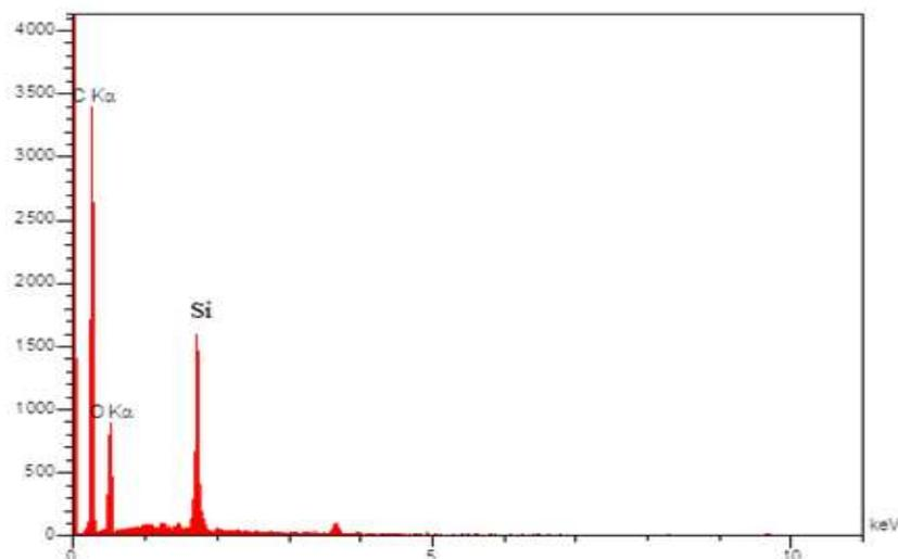
Fig. 3 EDX Spectrum of DLC film at 300mj
