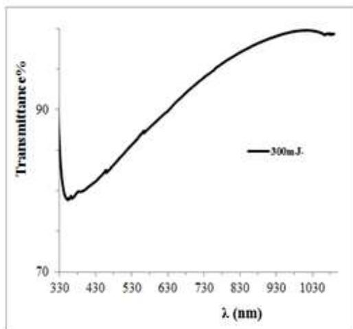
Fig. 5 Transmittance spectra for DLC film at 300mj
