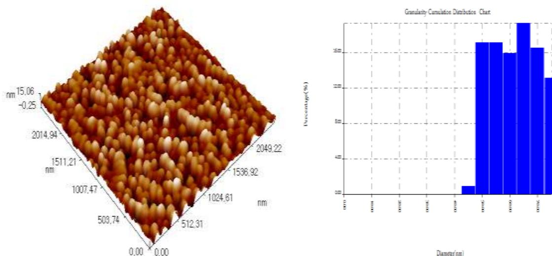
Fig.(4) 3D AFM image of the DLC (a) and grain size distribution (b)
