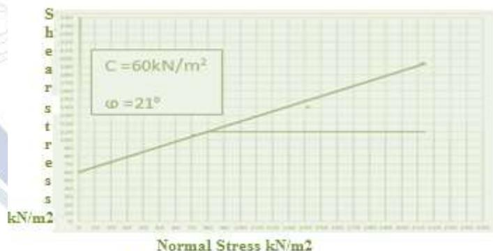
Figure 8: direct shear test site 1
