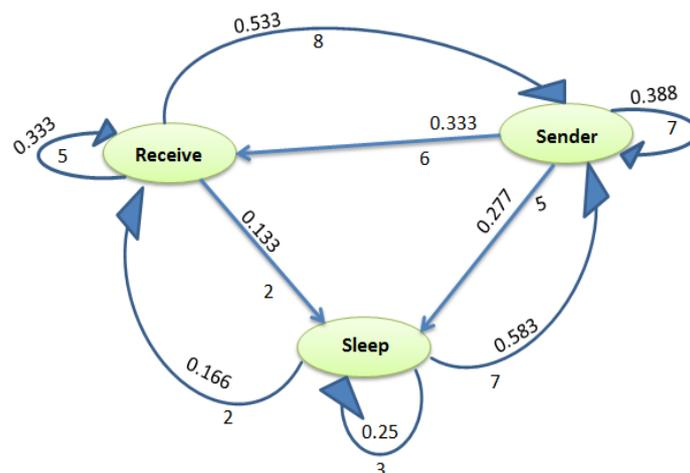
Figure 6: shows the switching states for node 6 and its states change probabilities.
