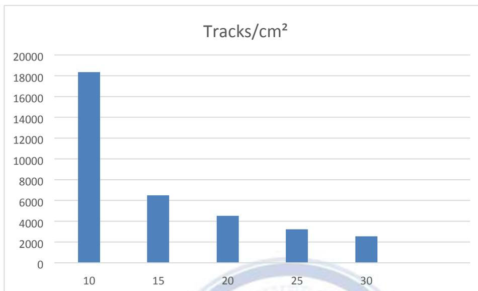
**Fig. (2) The density of track/cm<sup>2</sup> on the CR-39 according to the height of chambers**
