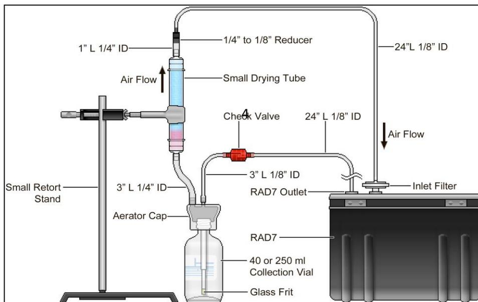
**Fig.(2) Schematic diagram of RAD7, solid state, ion implanted, planar silicon alpha detector with RAD H2O.**
