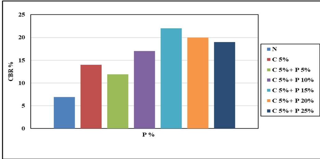
Figure 8: California bearing ratio values before and after adding improvement materials
