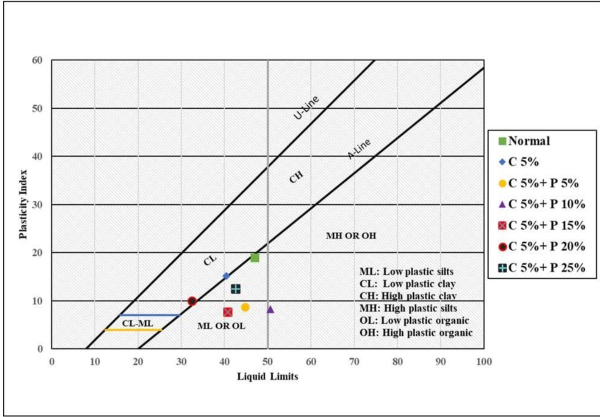
Figure 3: Values for cohesive soils' liquid limit and plasticity index both before and after the addition of improving materials are shown in the plasticity chart
