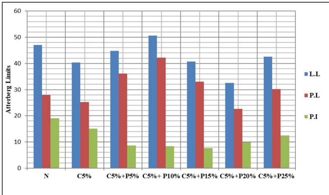
Figure 4: Atterberg's limits values for cohesion soil before and after adding improving materials
