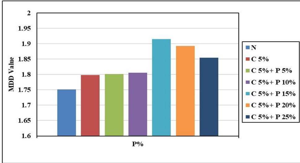
Figure 6: Maximum dry density values for cohesive soil before and after adding improving materials
