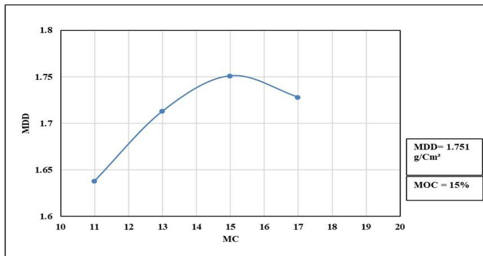
**Figure 5: Values of maximum dry density and optimum moisture content for natural cohesive soil**
