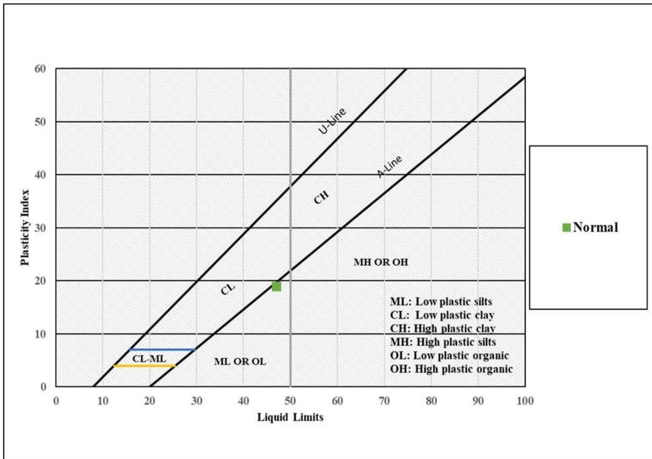
**Figure 2: The plasticity diagram displays the liquid limit and plasticity index values for naturally cohesive soil**
