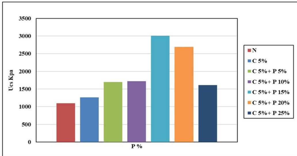
Figure 7: Unconfined cohesive soil compressive strength values both before and after the addition of improving materials
