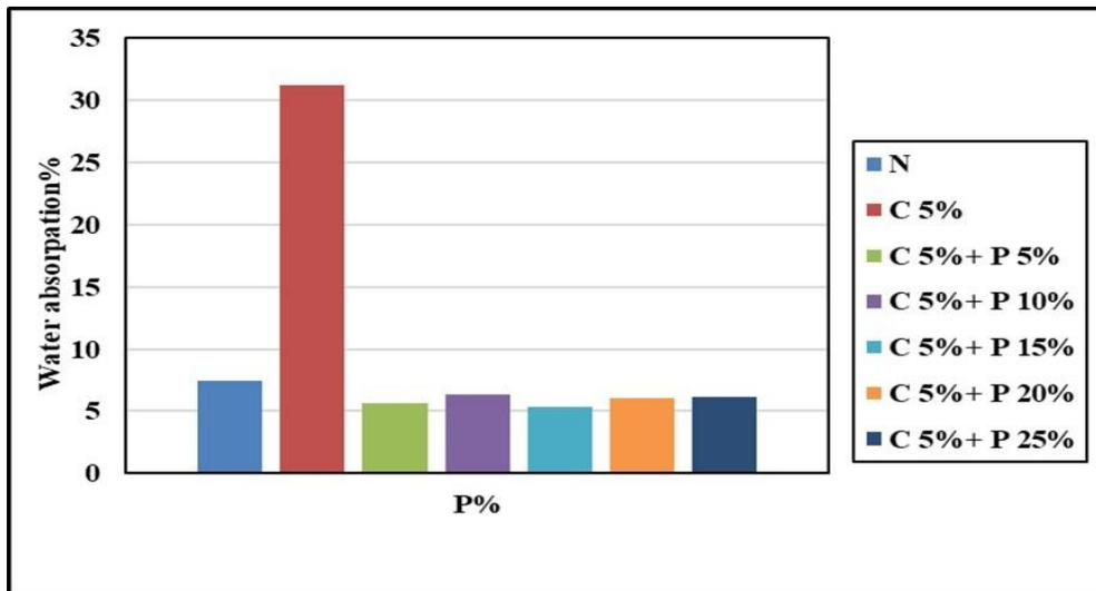
Figure 9: Absorption rate values for cohesive soil before and after adding improving materials
