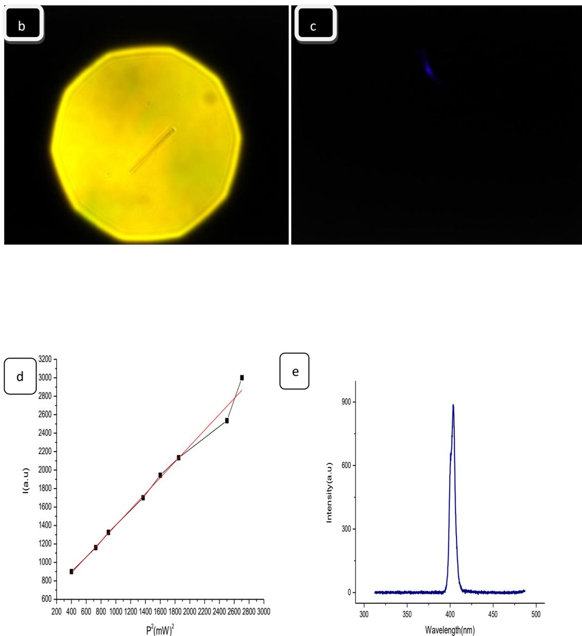
Figure 3 (a) shows the experimental setup schemes of the SHG optical measurement, (b) illustrates the bright – field image of the CdS nanobelt, (c) illustrates the dark–Field image of resulted SHG, (d) shows the spectral emission of the SHG using a pumping power of 20 mW (~31.8k W/ cm $^2$ ), (e) Shows the relation between power density of doubled frequency Ti:Sapphire irradiation and square value of power.
