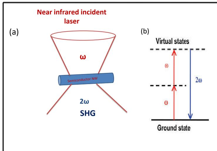
Figure 1) (a) Diagram of the SHG mechanism in semiconductor nanowire.
