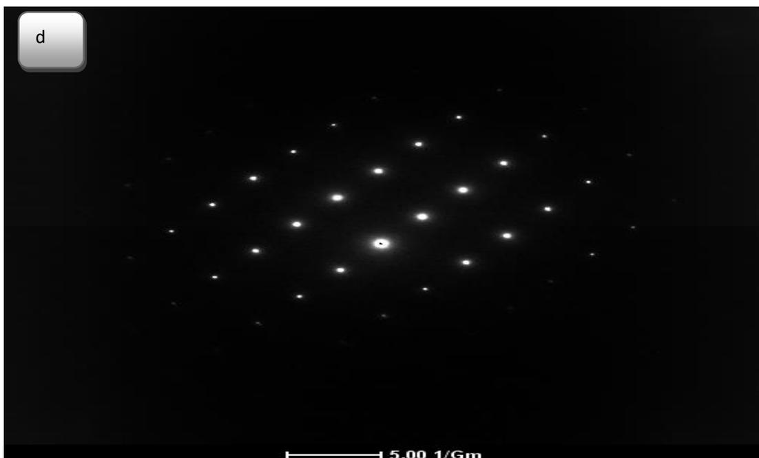
**Figure 2 (a) Low zoom image of SEM, (b) High SEM image magnification, (C) Low-zoom image of TEM, (D) is the corresponding SAED pattern of CdS nanobelts.**
