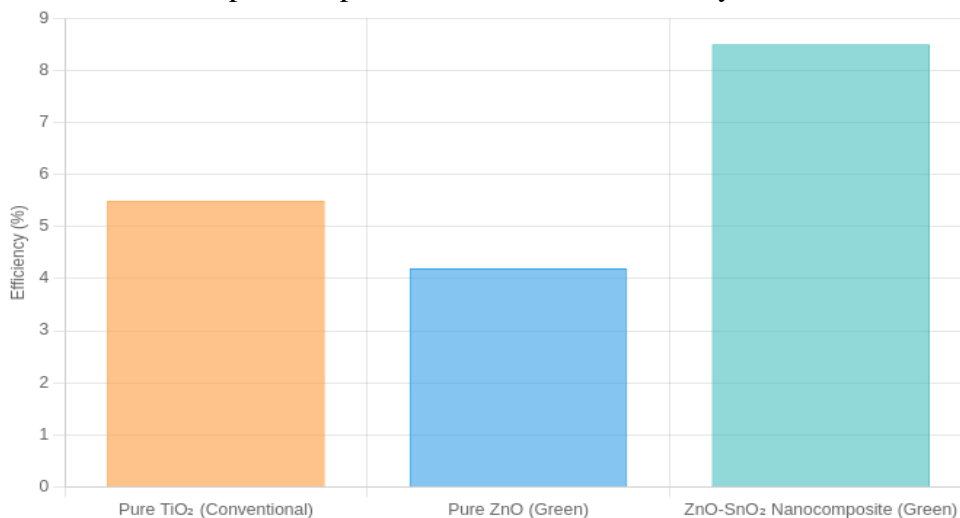
Figure 7. Anticipated Power Conversion Efficiency (PCE) of Dye-Sensitized Solar Cells (DSSCs) using different photoanode materials
