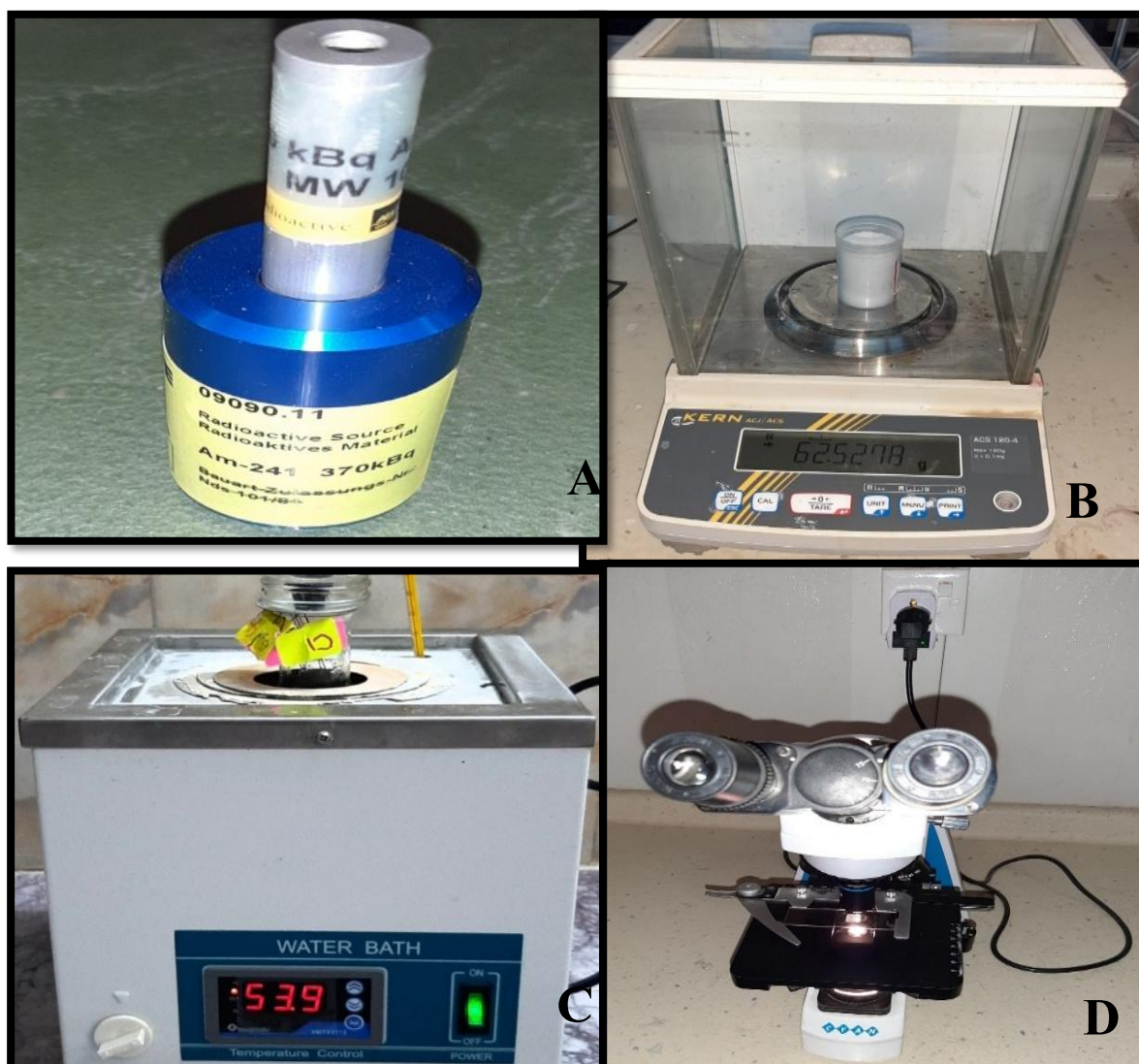
Figure (1) A indicates the radioactive source of alpha particles Am-241, while B indicates the sensitive balance. C the water bath etching device at different temperatures and D indicate the optical microscope to view the paths of ionized alpha particles in commercial detectors.
